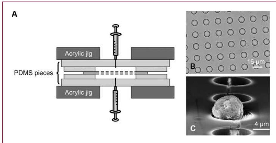
**Fig. 1.** Illustration of device assembly. A, schematic drawing of a functional microdevice consists of parylene membrane filter sandwiched between rectangular PDMS slabs and clamped in between acrylic jigs with inlet and outlet for syringes. B, bright field image of an optically transparent parylene filter with uniformly shaped and spaced 8- $\mu\text{m}$  pores. C, scanning electron microscope image of single cultured tumor cell captured on the membrane.
