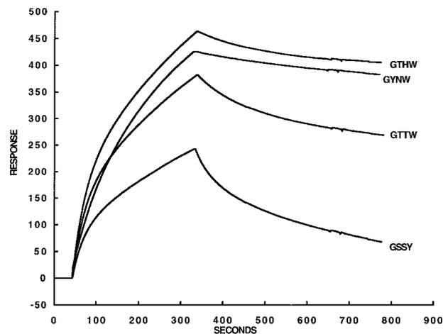
**Fig. 3** Biacore sensograms of RFB4(Fv)-PE38 mutants. Binding profile of WT immunotoxin GSSY is compared with mutants GTTW, GTHW, and GYNW. RITs were diluted to 25 μg/ml in HEPES buffered saline buffer and injected over a chip surface containing CD22. Binding kinetics were analyzed using BIA evaluation 2.1 software. *Y axis*, the resonance units bound. *X axis*, the time in seconds.
